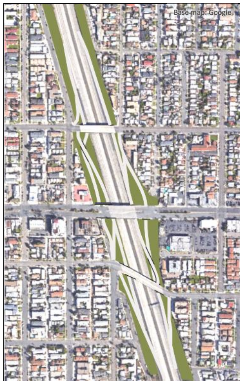
Figure 6.13 New I-805 Ramps The design goal of rebuilt freeway ramps is to permit freeway access to both Meade Avenue and Howard/Orange Avenues, while also allowing cars from these two roads to easily cut across to the other so as to facilitate movements in the east/west directions.
