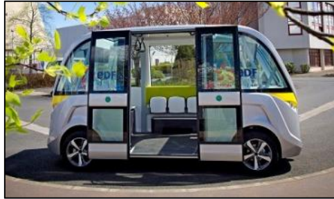
Figure 5.10 Automated Shuttle Small, automated, self-guided shuttles are now commercially available. They can bring large land areas within direct access of a station.
